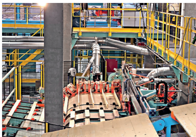
Mayr-Melnhof Holz uses Türmerleim's PU adhesive for the gluing of both surfaces and narrow edges
